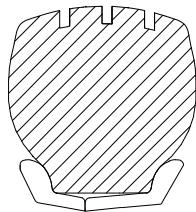
The wheelchair drive wheels have pneumatic tires or flat-free (foam filled) tires. The caster wheels have solid polyurethane tires.
