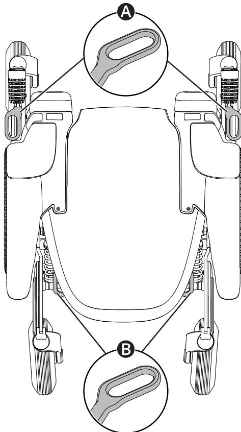
The wheelchair is equipped with four tie-down points used for transportation. Two in the front **A** and two in the rear **B**.
