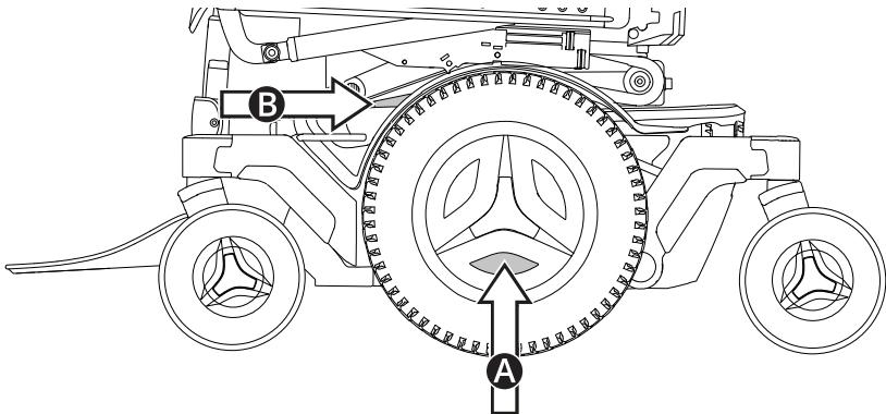
The serial number label is located on the lower, left side of the wheelchair chassis **A**. An additional serial number label is located on the seat tilt **B**. You may need to tilt the seat to see the serial number label.
