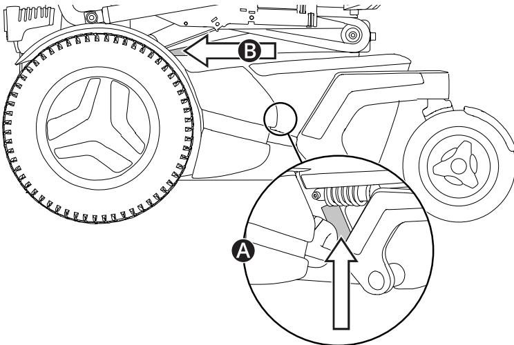
The serial number label is located on the lower, left side of the wheelchair chassis **A**. An additional serial number label is located on the seat tilt **B**. You may need to tilt the seat to see the serial number label.
