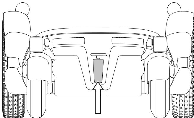
The wheelchair is equipped with reflectors at the front and rear.
