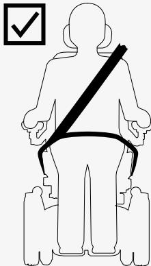
The shoulder-belt restraint should be worn over the middle of the shoulder. The pelvic-belt restraint should be in contact with and worn low across the pelvis and within the preferred zone of 30° to 75°. A steeper pelvic-belt angle between 45° to 75° to the horizontal is preferred. Make sure that no components of the wheelchair are lifted or tilted. The wheelchair must be in the position shown in the image.
