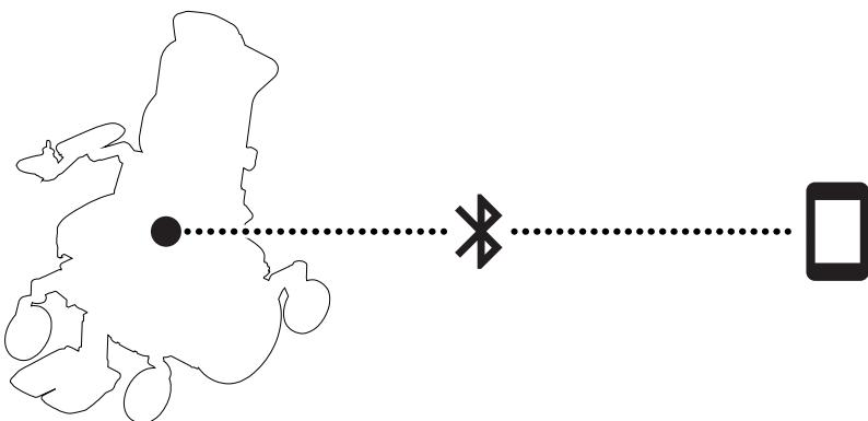
ConnectMe contains a radio transmitter. In certain areas, radio transmission is not allowed and ConnectMe must be set to flight mode ✈.
