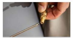
To quickly deflate the cushion, use the hand tool supplied to remove the valve core. Then apply pressure to the cushion by hand or by sitting in the chair until the cushion is fully deflated.
