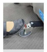
**To Brake Castor** using your foot, push lever down
