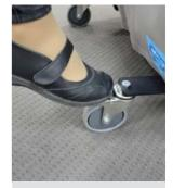
**To Unbrake Castor** using your foot, push top of lever down
