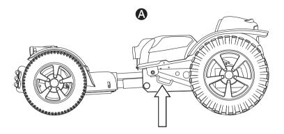
The wheelchair is equipped with four tie-down points used for transportation  $\blacksquare \checkmark \blacksquare$ . Two on the sides O and two at the rear O.
