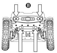
The wheelchair is equipped with reflectors at the front, the rear and the sides. It is also equipped with front lights, rear lights, and indicators.
