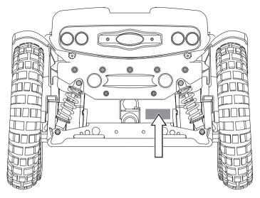
The serial number label is located on the rear of the wheelchair chassis.
