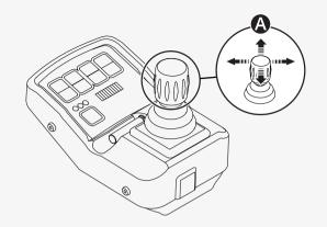
Turn off the power before you get in or out of the wheelchair or lift the armrest. Do not use the joystick as support when you get in or out of the wheelchair.
