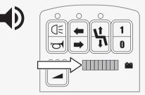
Seat rotation out and seat lift pinch protection active Error code: LED 3 flashes. If pinch protection is active, the seat lift cannot be lowered. If the seat rotation is out, the wheelchair cannot be driven.
