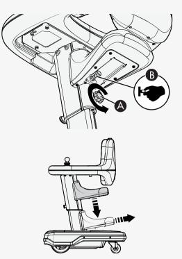
5. Put back the tightening knob and tighten it by hand.
