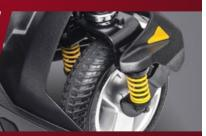
Comfort-Trac front and rear suspension for added comfort. The Go-Go<sup>®</sup> LX with Comfort-Trac Suspension (CTS) offers a whole new level of comfort and performance. This industry-first CTS technology incorporates advanced suspension for improved absorption over various terrains. The Go-Go LX with CTS offers a 300 lb. weight capacity, a per charge range up to 8.6 miles and a maximum speed of 4.4 mph.
