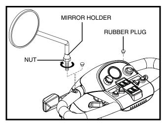
Figure 14. Mirror Installation and Positioning
