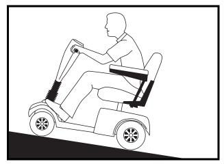
Figure 2A. Increased Stability Driving Position
