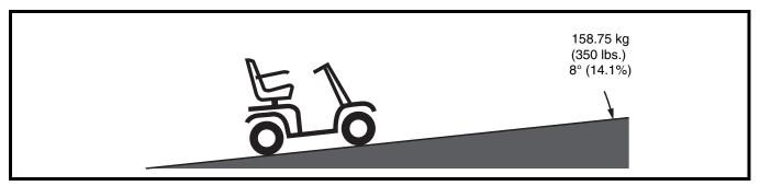
Figure 1. Maximum Recommended Incline Angles
