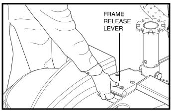
Figure 20. Frame Release Lever
