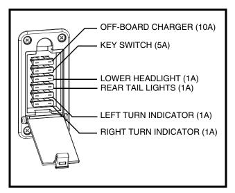
Figure 6. Tiller Console Fuses
