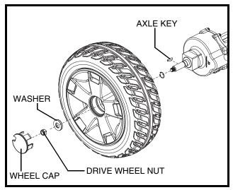
Figure 22. Solid Tire Wheel Removal
