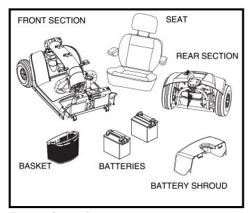
Figure 18. Scooter Components
