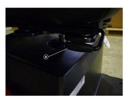
You can adjust the amount of legroom on the scooter by sliding the seat back and forth. To slide the seat, lift up the seat sliding handle (B). Located on the right of the seat. Then adjust the seat to correct position, release the handle and continue sliding the seat until it locks in position.
