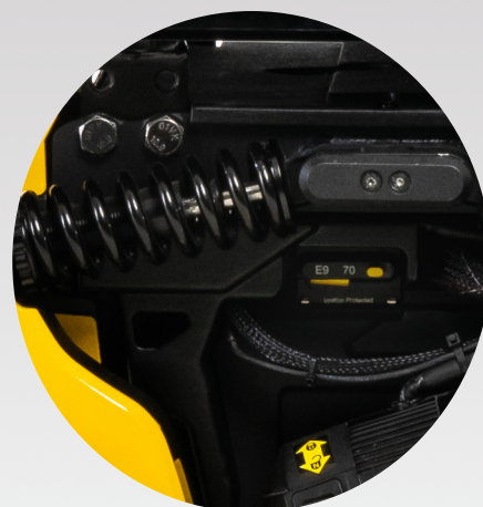
INTEGRATED BATTERY ISOLATION SWITCH
