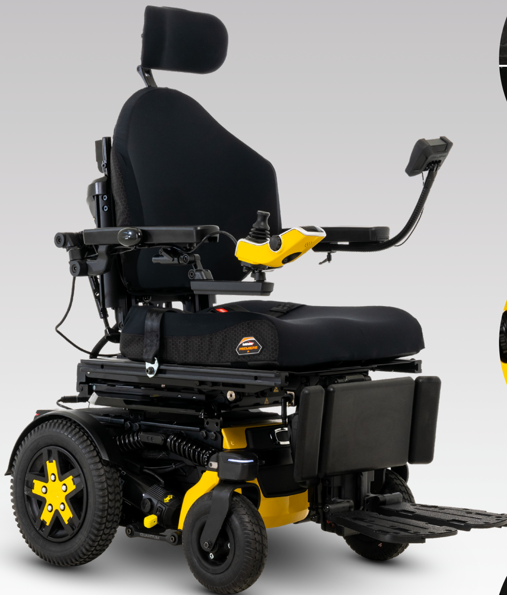
FRONT LIGHT INTEGRATED INTO THE CASTER ARM
