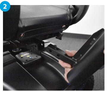
Take the Walking stick holder and insert the connector in to the rear receiver on the scooter
