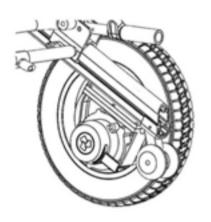
Do not operate clutch handle by foot, it would probably damage the brake.
