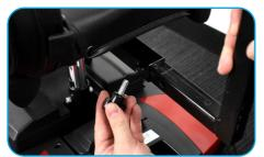
1 Place L shaped bar in rear receiver of scooter and place metal pin and/or screw in position.
