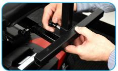
3 Slide the small T shaped bar to the very bottom of the L shaped bar and tighten screw into position.
