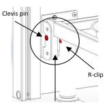
The clevis pins and R-clips locked position
