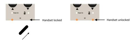
The handset is locked when the bed just has a power supply.
