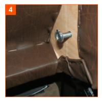
Fit screws securing the backrest brackets on the inside of the backrest.
