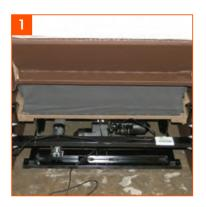
Line backrest up as close as possible to the backrest brackets (it may sometimes be necessary to bend the brackets on the mechanism inwards slightly).
