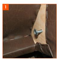
From the inside of the backrest, remove the screws securing the backrest brackets.
