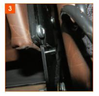
Carefully push the backrest down into place until the backrest bracket hits the stopper on the mechanism bracket taking care to make sure the backrest remains square and upright.
