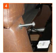
Retighten the screw at the back of the armrest.
