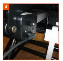
Connect the new handset plug into control box.
