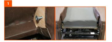
Remove backrest – remember to remove the screws securing the backrest brackets on the inside of the backrest
