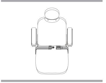
Figure 13. Positioning Belt Adjustment
