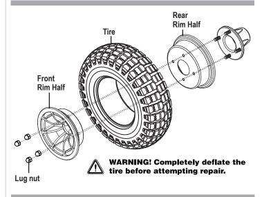
Figure 17. Drive Wheel Disassembled
