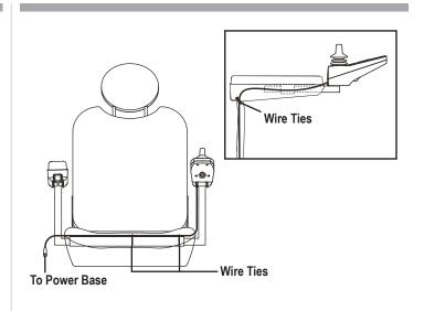
Figure 7. Controller Harness Routing on a Contour Seat
