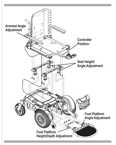
Figure 3. Assembly View (Synergy Seating System Shown)
