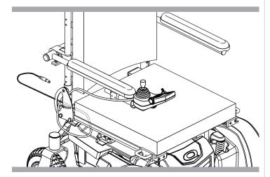
Figure 6. Controller Harness Routing on a Synergy Seat
