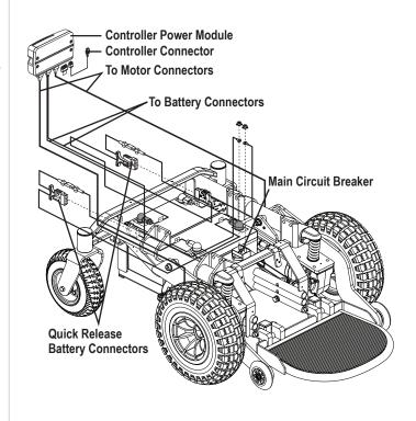
**Figure 1. Electrical Components**
