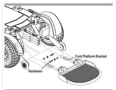
Figure 12. Foot Platform Adjustment
