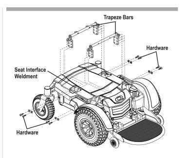
Figure 9. Seat Height/Angle Adjustment
