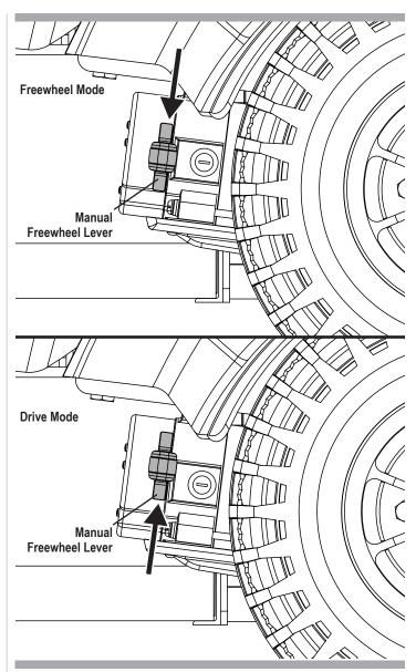
Figure 2. Manual Freewheel Lever Operation
