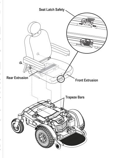
Figure 4. Universal Mounting System and Contour Seat
