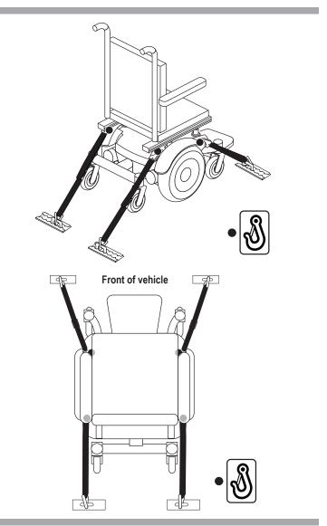
Figure 8. Unoccupied Transit System Securement Points
