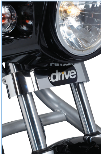
Telescopic front motorcycle suspension for optimal handling
