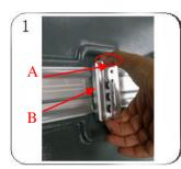
To open press button (A), (near keyhole) then pull bottom of the latch (B)
