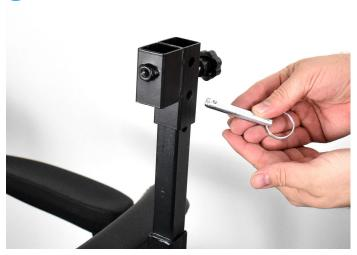
Secure with bolt and metal pin
