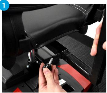
Place L shaped bar in rear receiver of scooter and place securing rod or screw bolt in position.
