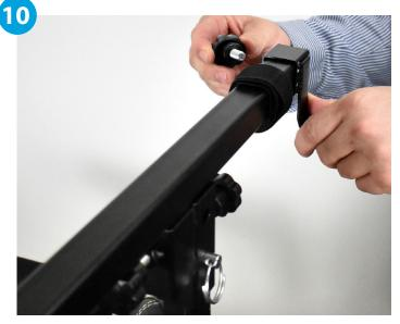
Bolt the right-side hanging clip into position facing outwards at the end of the T piece bar
