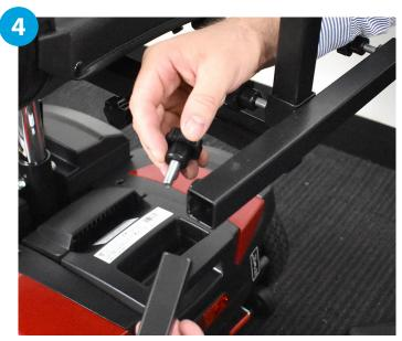
Place small extension bars at both ends of the T shaped bar and fasten with bolts
