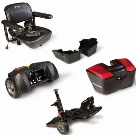
One-hand "Feather Touch" disassembly
