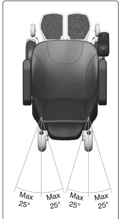
The angle of the rear fastening straps may not exceed 25°.
